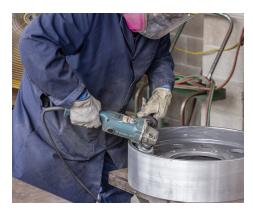
Our expert technicians carefully strip, clean, polish and inspect the cores for refurbishing.
