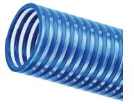
TIGERFLEX SOLARGUARD HIGH UV RESISTANCE PVC SUCTION HOSE Construction: PVC tube with rigid PVC helix Temperature Range: -4°F (-20°C) to +150°F (+65°C) Typical Application: Irrigation and liquid fertilizers. Blue Clear 3/4"-4" & Solar Guard 1-1/2 & 2" in stock
